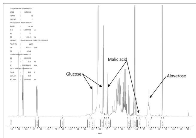
Figure 1 - <sup>1</sup>H-NMR spectrum of *A. vera* gel material.
