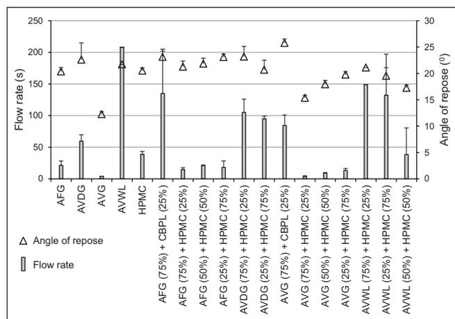
**Figure 3** - Angle of repose and flow rate of the individual powders and mixtures of powders. Values represent the average  $\pm$  standard deviations (error bars) of three replicates.
