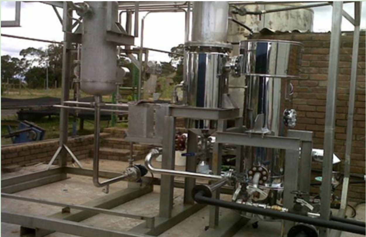
Alcohol distillation plant for producing A. ferox inner leaf gel Source: Mr Chris Pattinson, Organic Aloe
